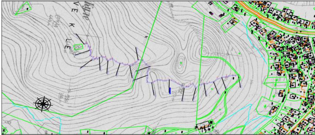
Picture 15: Marked route for construction of access trail with candelabras and foundation
