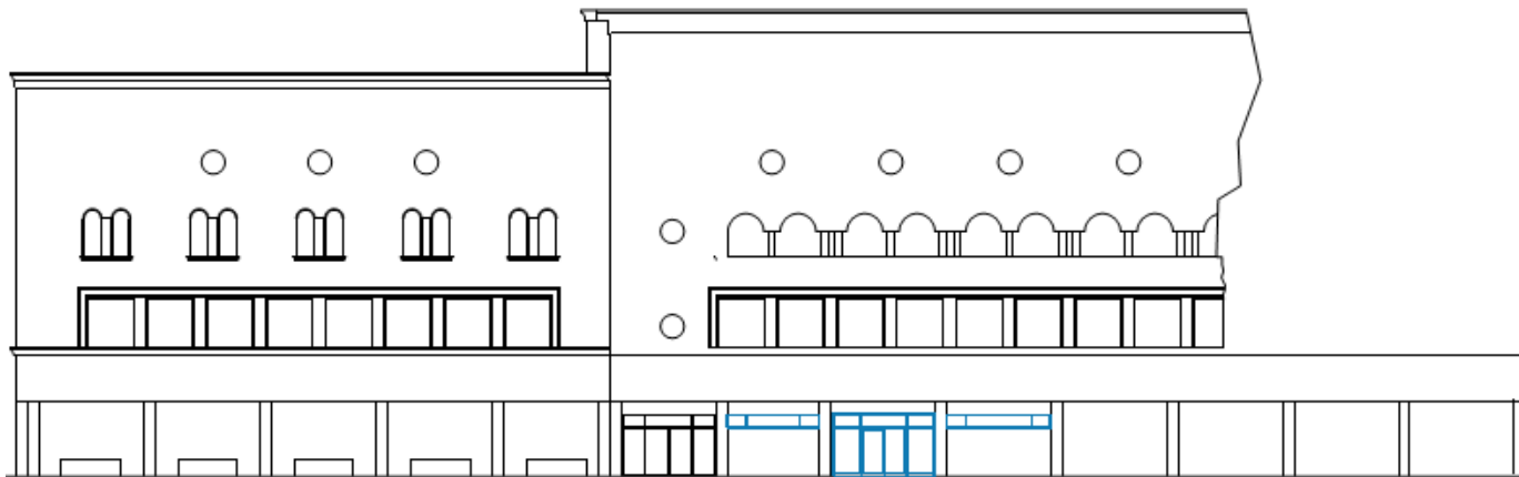
Figure 14 Newly designed situation southern façade (with blue color are shown location of new windows and doors)
