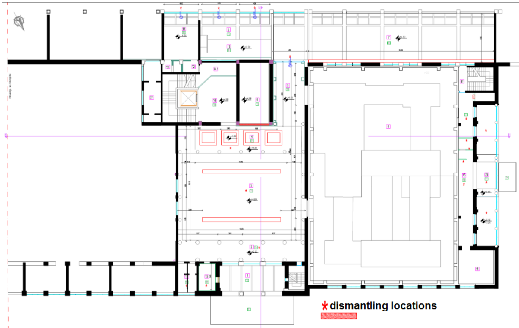
Figure 4 Base view of the ceiling of the ground floor (currently) with marked dismantling locations
