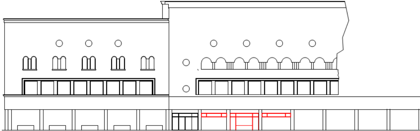
Figure 13 Current situation southern facade (with red color are shown dismantling locations)
