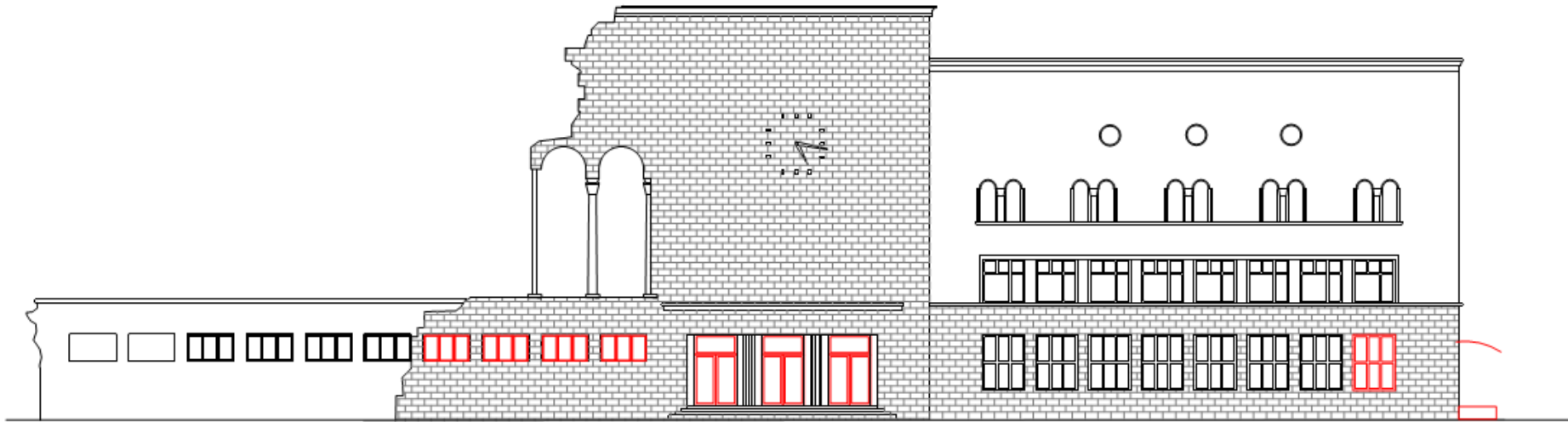
Figure 11 Current situation north facade (with red color are shown dismantling locations)
