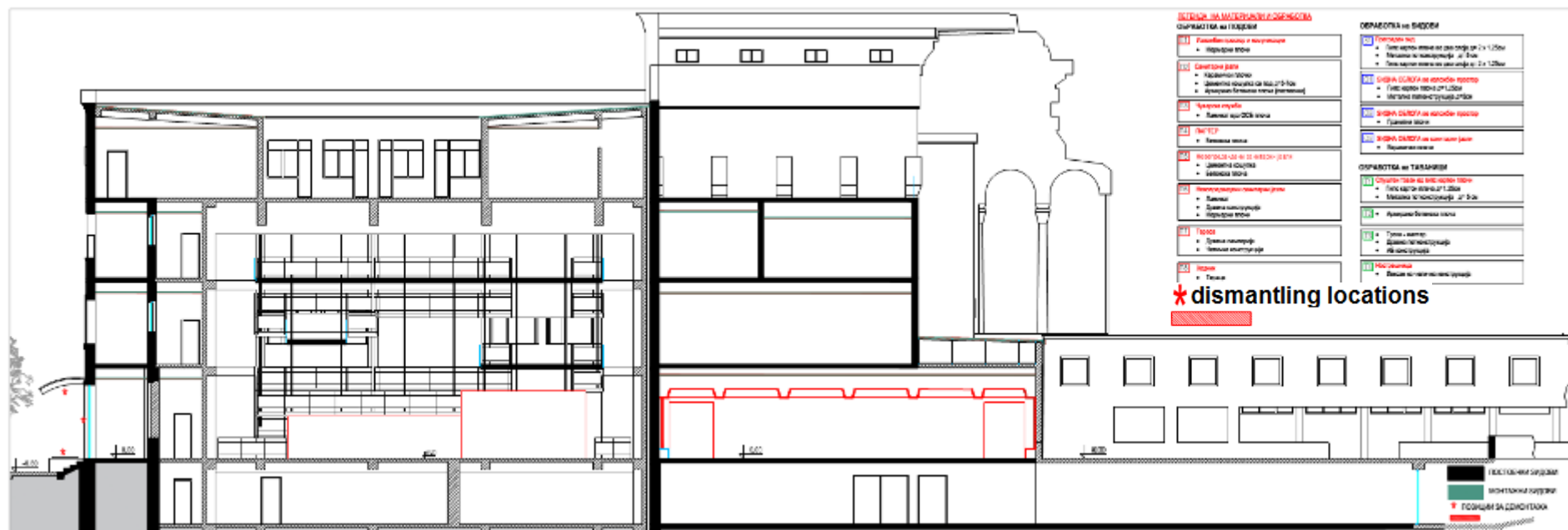
Figure 9 Current situation cross-section B-B with marked dismantling locations
